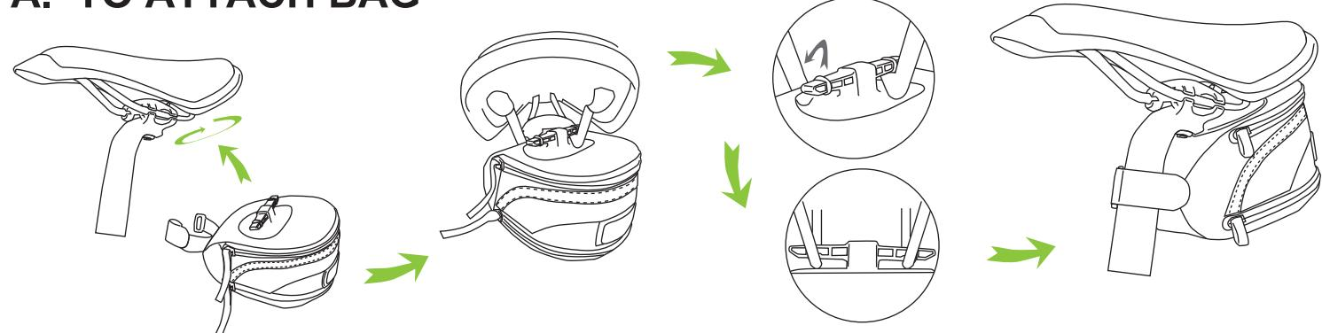
(1). Insert one end of plastic T-Bar into saddle rail.
