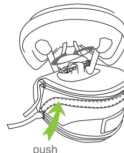
(2). Push T-Bar to one side and then twist T-Bar to release from rails.
