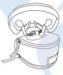
4 · Secure saddle bag to seat post by using Velcro strap
