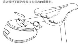
3 · Adjust the T-bar buckle until the both ends are even. 請調整T字型扣具至平穩的狀態。
