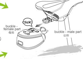
$3 \cdot \text{To remove the saddle bag, squeeze the two sides of}$ the female part of buckle and pull the bag off. 按壓母扣突出的兩側, 即可將袋子卸除 按压母扣突出的两侧, 即可将袋子卸除
